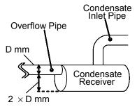
Vented Receiver Table- 1 (For atmospheric, open system installations)
