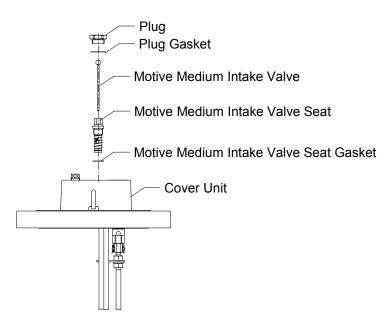
NOTE: It is possible to remove and replace the intake valve (motive medium) without first removing the cover of the PowerTrap (see instructions above).
